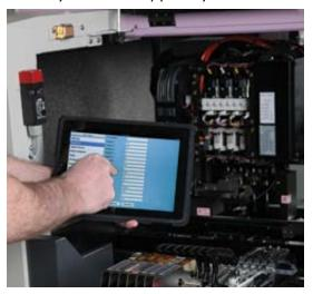
your hand! CTC qMon is based on Control Technology Corporation's CTC Monitor Utility. Simply enter your controller's IP address to wirelessly connect to it. Once connected, the app presents the current status of the target controller's:
