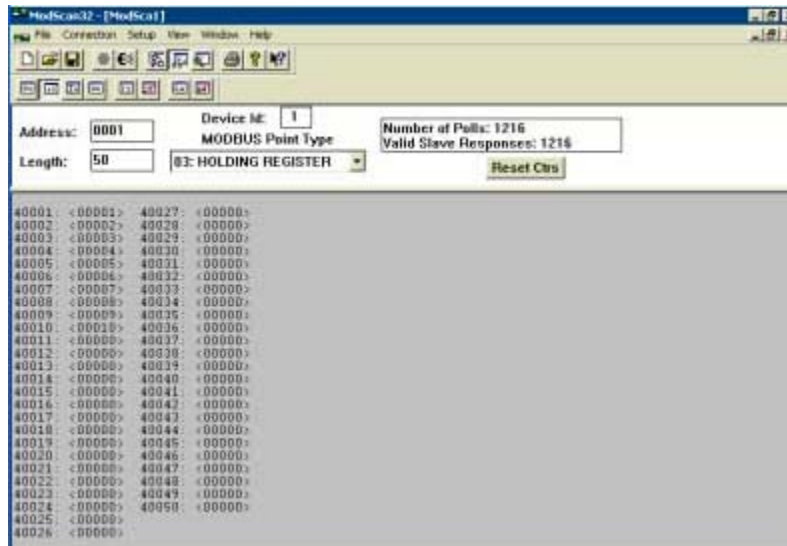
Figure 1.10: New values written and read back, Quickstep registers 1 to 5, Modbus 1 to 10
